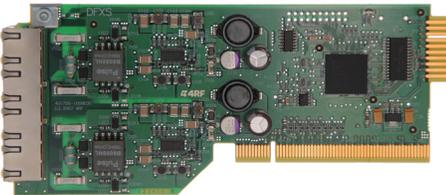
The function of FXO / FXS two wire loop interface circuits is to transparently extend the 2 wire interface from the exchange line card to the telephone / PBX, ideally without loss or distortion. These circuits are known as 'ring out, dial in' 2 wire loop interface circuits. The DFXS interface simulates the function of an exchange line card.
