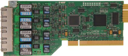
The Q4EM is a quad port analogue interface card providing a 4 wire analogue circuit and single E&M signalling.
