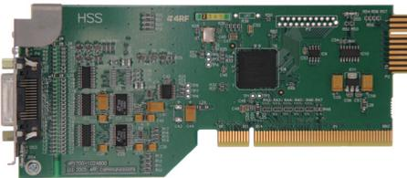
The HSS is a single port high speed serial interface card providing V.35, X.21, RS-449 and RS-530 synchronous data transmission as either a DTE or a DCE. It supports data rates of 8 to 2048 kbit/s in 8 kbit/s steps (dependent on rate selected). 8 kbit/s is used for control lines.
